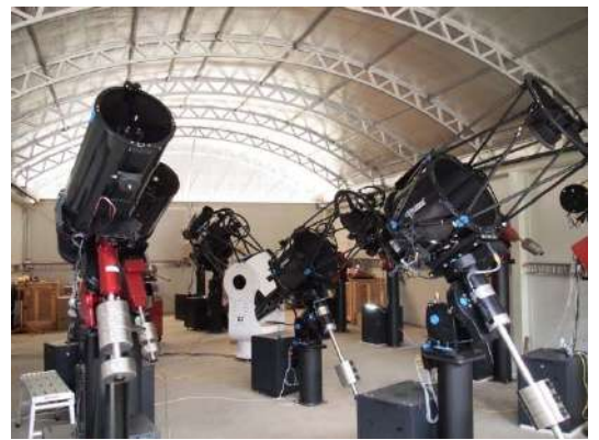
Figure 80 - The interior of the iTelescope building, showing the truss roof which slides off entirely to permit viewing through the remotely operated telescopes it contains (Context 2014).
