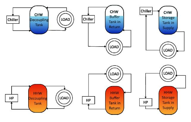
Figure 1: Storage tank hydraulic connection details, HP=heat pump, CHW=chilled water, HHW=heating hot water
